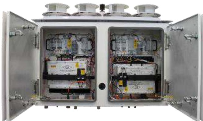
Figure 4 - Transceiver enclosure for mast / tower mounting
