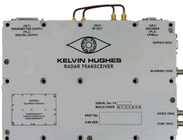
SharpEye™ transceiver located in upmast turning unit housing
