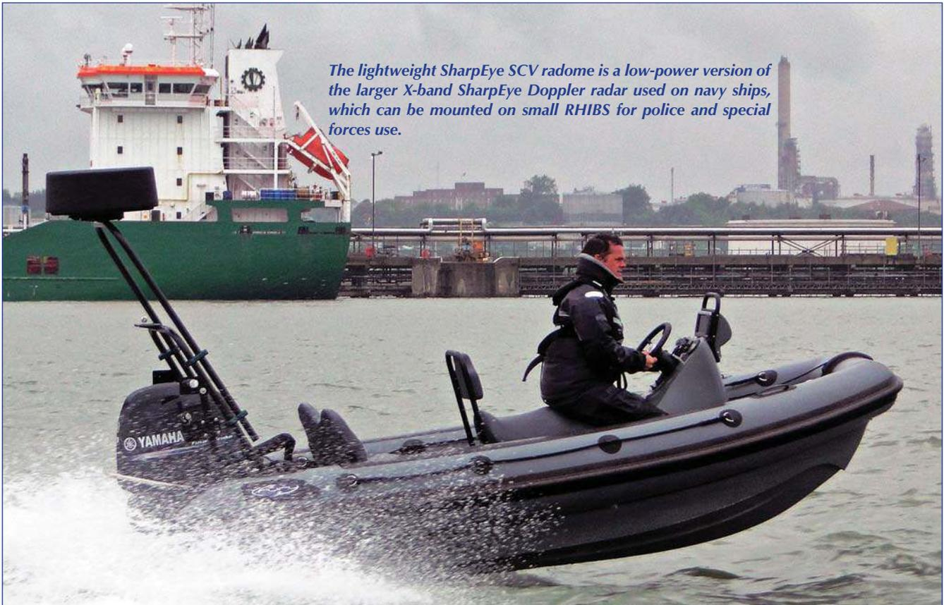
*The lightweight SharpEye SCV radome is a low-power version of the larger X-band SharpEye Doppler radar used on navy ships, which can be mounted on small RHIBs for police and special forces use.*
